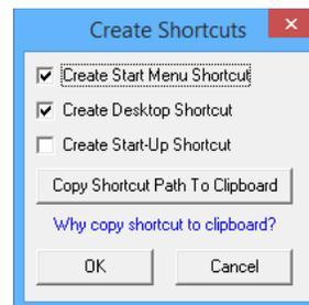
If you intend to launch ScadaPhone via some other means (e.g. a script command executed by the SCADA software), you can obtain the path to the **Start Menu** shortcut (**.LNK** file) by clicking the **Copy Shortcut Path To Clipboard** button.
