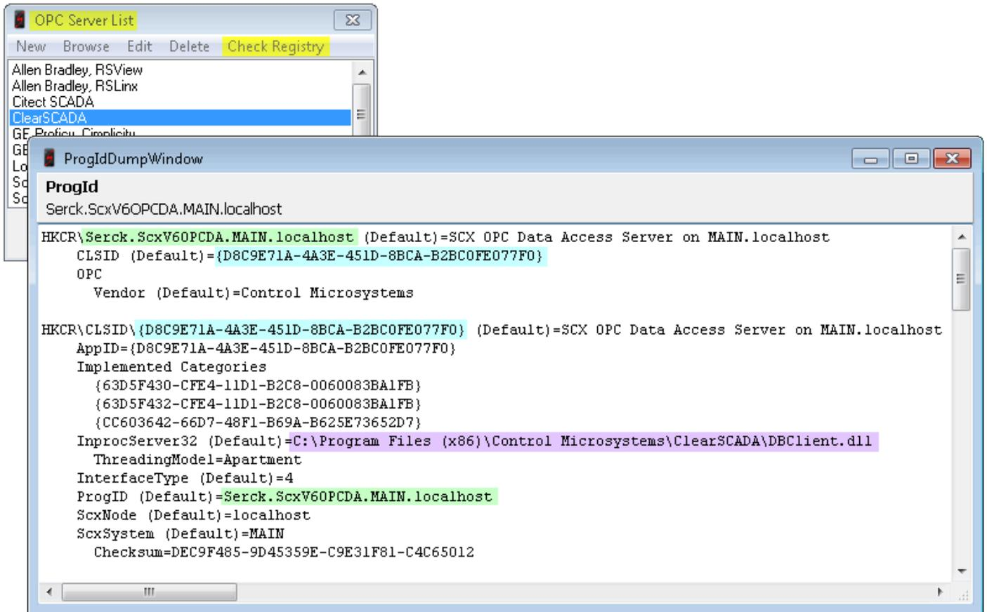
The image above shows the results of doing the **Check Registry** operation on a computer where **ClearSCADA version 6** is installed. Older versions of ClearSCADA used the **Serck.ScxV6OPCDA.... ProgID**, but newer versions of ClearSCADA require a different **ProgID: ControlMicrosystems.KEPServerEX**
