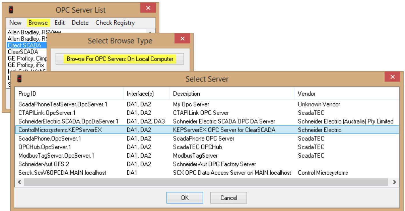
After selecting the new **KEPServerEX Prog ID**, ScadaPhone's **ScadaLink Setup** should look like this:
