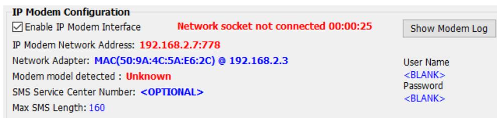
If there is a modem connectivity problem, ScadaPhone will also announce: *"I.P. modem network connection error"* over the local host-computer soundcard (when in **Run Mode**). If an **IP Modem Error Tag** has been configured into ScadaPhone's optional **Watchdog Features**, an alarm can be reported via some other reporting method (aside from the non-functioning IP Modem reporting method).
